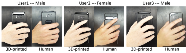
Figure 11: Illustration of the 3D-printed hand replay attack.
