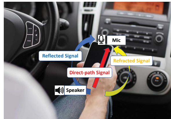
Figure 1. Illustration of the acoustic signal interacting with the driver's hand.
